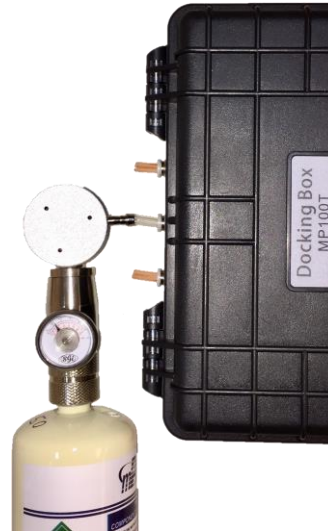
Calibration Gas Connections
